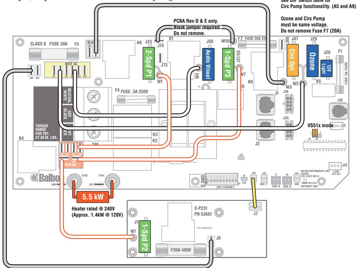
**WARNING:** Main Power to system should be turned OFF BEFORE adjusting DIP switches.
